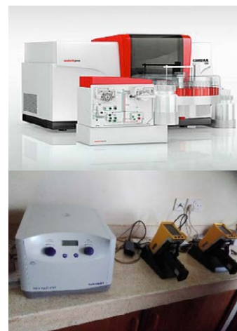
AAS machine for testing fertilizer quality including concentration of heavy metals
