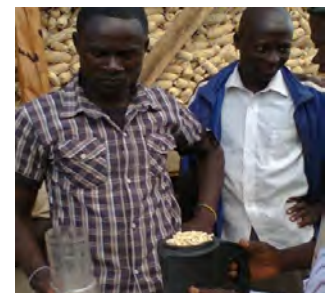
Testing MC using a moisture meter
